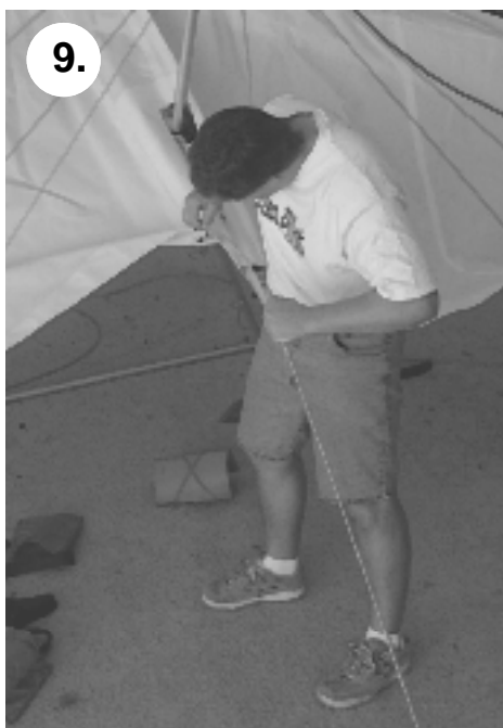
8. Insert the Kingpost over the nylon spacer and between the Pullback Cables . Note: when pulling the cables back, check to make sure they are not crossed or twisted.
